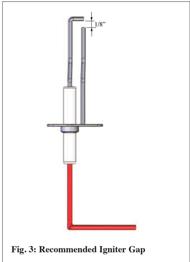
**Fig. 3: Recommended Igniter Gap**
