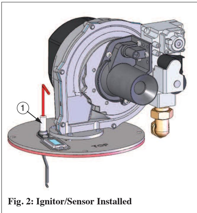
**Fig. 2: Igniter/Sensor Installed**
